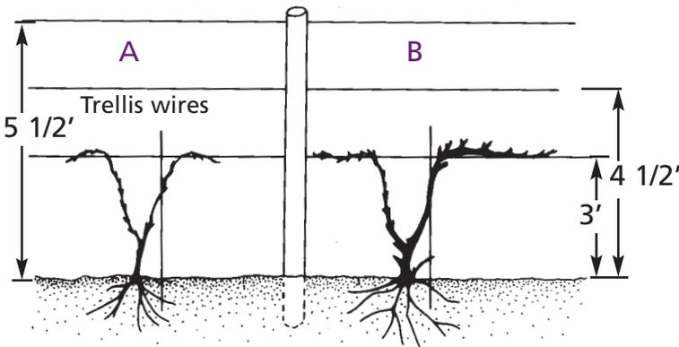
Figure 12. Bilateral cordon training system for grape vines, year three. (A) Spring, weak vine after pruning; (B) spring, vigorous vine after pruning.
