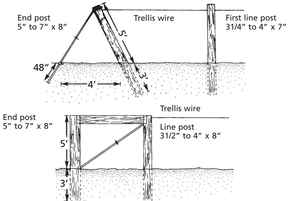
Figure 8. Dimensions for the end post construction for a grape trellis that can be used for either mid-wire or high-wire cordon training systems.
